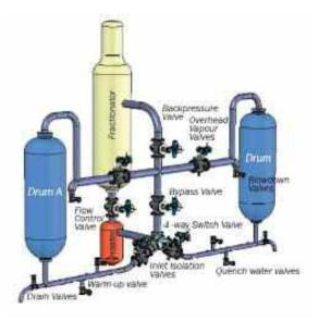
The delayed coker unit has two large vertical coker drums. During operation, one will be in coking service while the other is being decoked with high-pressure water jets. Steam removes residual hydrocarbons. The coke left in the drum is cut into fragments and carted away to coke storage or loading facilities.
